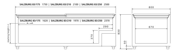
For version AD/U the inner dimensions are reduced due to the necessary use of wire grids along the inside walls.
