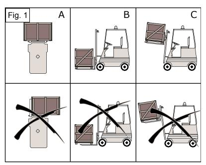
The package must be lifted by inserting the forks of the lift truck into the space between the legs of the pallet or crate. The weight of the equipment must be divided so that the centre of gravity of the package remains balanced (Fig.1-A). Do not tip the equipment over.
