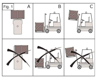
The package must be lifted by inserting the forks of the lift truck into the space between the legs of the pallet or crate. The weight of the equipment must be divided so that the centre of gravity of the package remains balanced (Fig.1-A). Do not tip the equipment over.
